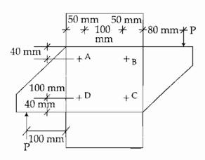
If all bolts are equal in diameter, which bolts are critical?
