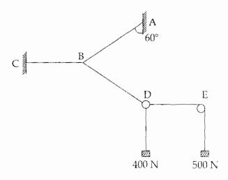
'D' is a weightless ring 'E' is a frictionless pulley. Calculate tension cable AB
